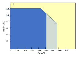
The darker blue area of the graph opposite represents the safe operating zone for this material. The light blue area should be tested, especially if there is high temperature steam present. The yellow area is generally outside safe working parameters.
