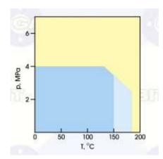
The graph opposite represents the safe operating zone for this material, basically within temperatures up to 150°C and pressures up to 4Mpa.
