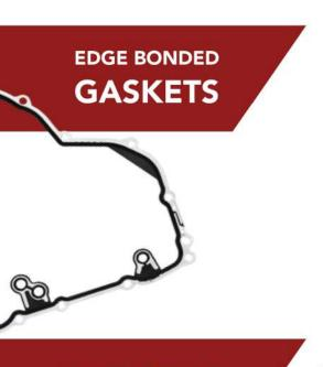
Designed to seal flat components, edge bonded gaskets comprise an elastomeric sealing bead that is bonded to the thin edge of a metal carrier frame. They are used to seal flat components when a groove is missing for a press-in-place gasket.
